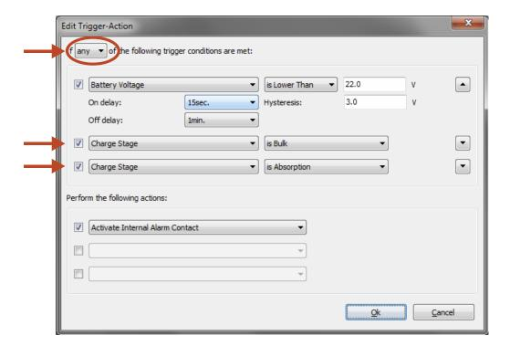
These settings make sure that as long as the charger is operating in the Bulk or Absorption stage, the charge process is still running, so the Trigger must remain active.
