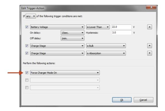
As you can see, we have selected 'Force Charger Mode On' to enable the charger while the any of the three Trigger conditions are met.
