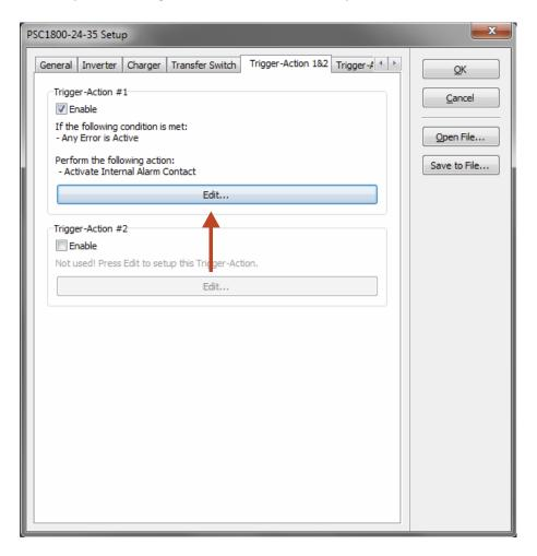
When you wish to keep the factory default Trigger-Action in place, you can also Enable Trigger-Action #2 and perform the steps below in the #2 Trigger-Action slot, by pressing the Edit button in this box.
