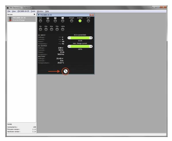
We need to press on the wrench tool button as indicated by the red arrow to activate the setup window. Please note that DIP switch no. 1, inside the Powersine Combi, needs to be set to ON (External programming). Otherwise setting up the Combi by the Dashboard software is blocked.
