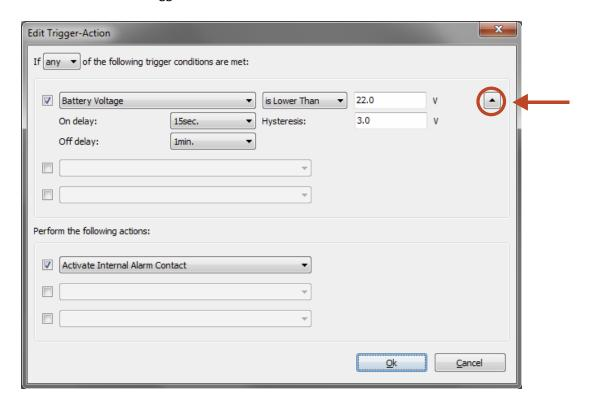
As you can see, we have set the 'On delay' to '15sec.', which means that the Trigger will be considered active once the battery voltage is lower than 22.0V for 15 seconds.
