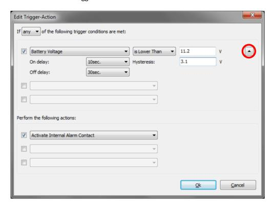
As you can see, we have set the 'On delay' to '10sec.', which means that the Trigger will be considered active once the battery voltage is lower than 11.2V for 10 seconds.
