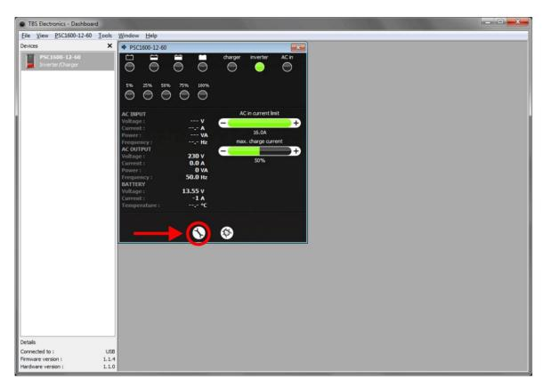
We need to press on the wrench tool button as indicated by the red arrow to activate the setup window. Please note that DIP switch no. 1, inside the Powersine Combi, needs to be set to ON (External programming). Otherwise setting up the Combi by the Dashboard software is blocked.
