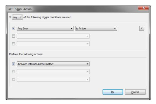
We will start by changing the Trigger conditions first. The trigger conditions in this example are: Start the generator when the battery voltage drops below 11.2V for 10 seconds and stop the generator again when the battery voltage is higher than 14.3V for 30 seconds (14.3V is 0.1V below the standard 14.4V absorption voltage of a 'flooded battery' charge program).
