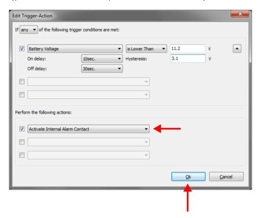
As you can see, we have kept the already existing Action to activate the internal alarm contact of the Combi once the Trigger conditions are met.
